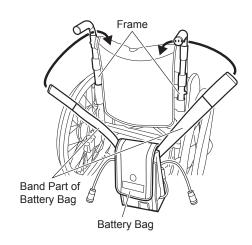
Case of Battery Bag Band Tip Part not Reaching to Battery Bag
