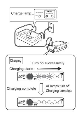
After charging has completed, unplug the charger plug and the power plug, then securely close the battery's connector cover.
