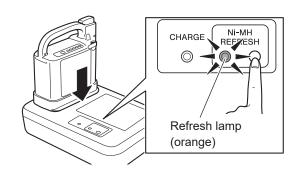
The refresh lamp (orange) changes from a flashing to an "on" state, and the refresh charging starts.
