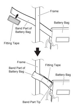
Case of Battery Bag Band Tip Part Reaching to Battery Bag
