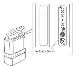
(2) Once the battery runs out, the warning lamp turns on, and a long buzzer beeps "Pi—" once and stops.
