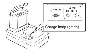
• The battery temperature increases during charging. However, if the battery temperature rises above 50°C (122°F), the power for the charger will turn off to protect the battery.
