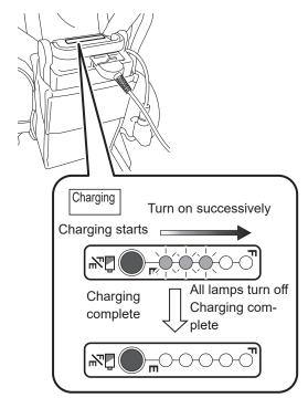
After charging has completed, unplug the charger plug and the power plug, then securely close the battery's connector cover.
