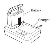
**TIP** After plugging in the charger, it takes about 5 seconds for the charging lamp to light.
