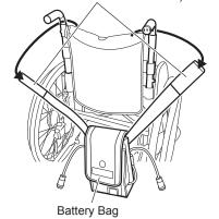
(5) Remove the hook-and-loop fastener of belt and remove the belt.
