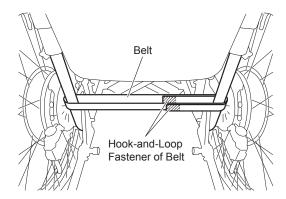
(6) Feed the belt through the frame under back support and attach the hook-and-loop fastener.
