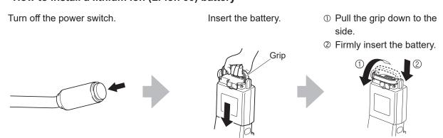
Please open the Battery-bag and insert the Battery into the bag in the same manners as that of Ni-MH Nickel Metal Hydride Battery. After inserting please pull down the grip so that the battery is firmly inserted to the position.
